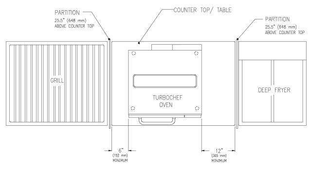
FIGURE 5: Installation Near Open Heat Source
