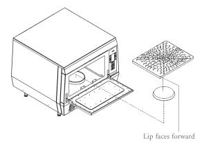
FIGURE 3: Oven Assembly and Ceramic Platter Installation
