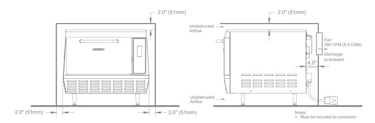
FIGURE 4: Built-in Installation
