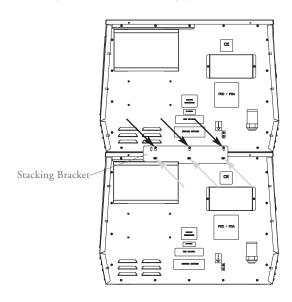
FIGURE 1: Double Stacking Ovens
