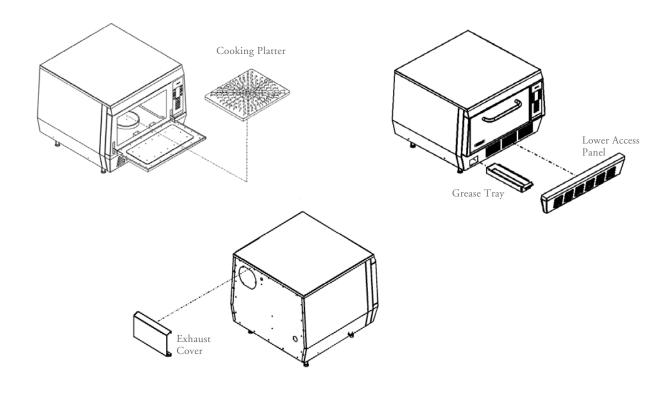
FIGURE 20: Removing Components for Cleaning.
