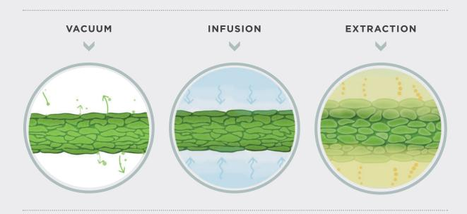
Vacuum removes the air from the cells
